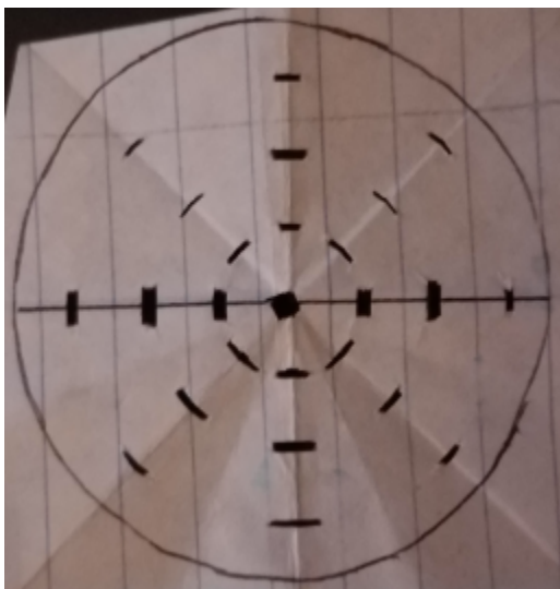
Figure 1. The grid template is 5.5 cm diameter circle, the same size as the petri dishes used. A box was made in the center. The eight boxes immediately surrounding the center box comprise Zone 1. The eight boxes immediately surrounding Zone 1, comprise Zone 2. The eight boxes immediately surrounding Zone 2, comprise Zone 3. From the center box each box in Zone 1 is 0.75 cm in distance. Zone 2 boxes are 1.5 cm away from the center box and Zone 3 boxes are 2.25 cm away from the center box.
